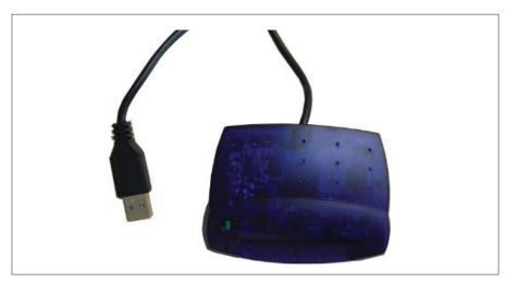
The CP 6000 Chip Card Programmer/ Reader is used for programming and reading CC 6010 Chip Cards. The CP 6001 is connected to a USB port on the PC running the SW 6000-CAA Application with the SW 6071 Module: "Chip Card Programming" enabled.
