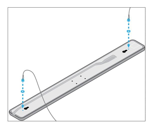
3. Thread the cable ends through the 2 Gripple connectors as shown. Squeeze the sides of the Gripple connector to adjust the cable's length. Trim excess cable, leaving at least 1 inch (25 mm).
