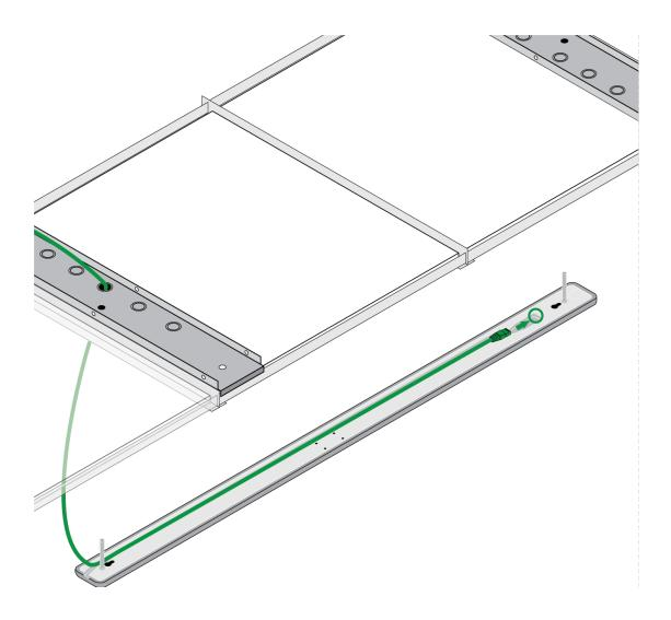
3. Push the bolts through the holes in the ceiling tiles to place the microphone on the ceiling. Hold the microphone in place and attach the wing nuts and washers to the bolts.
