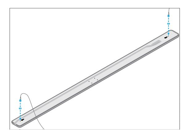
3. Thread the cable ends through the 2 Gripple connectors as shown. Squeeze the sides of the Gripple connector to adjust the cable's length. Trim excess cable, leaving at least 1 inch (25 mm).
