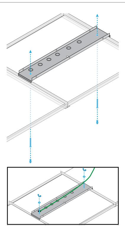
2. Attach the eyelets, cable, and M5 washers to the MXA710.
