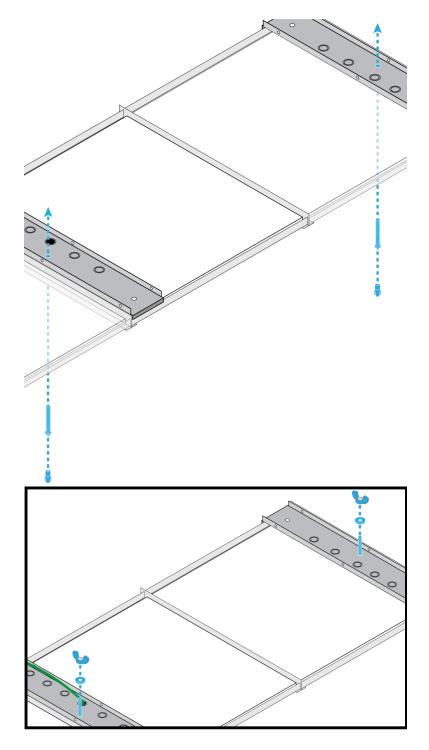
2. Attach the eyelets, cable, and M5 washers to the MXA710.
