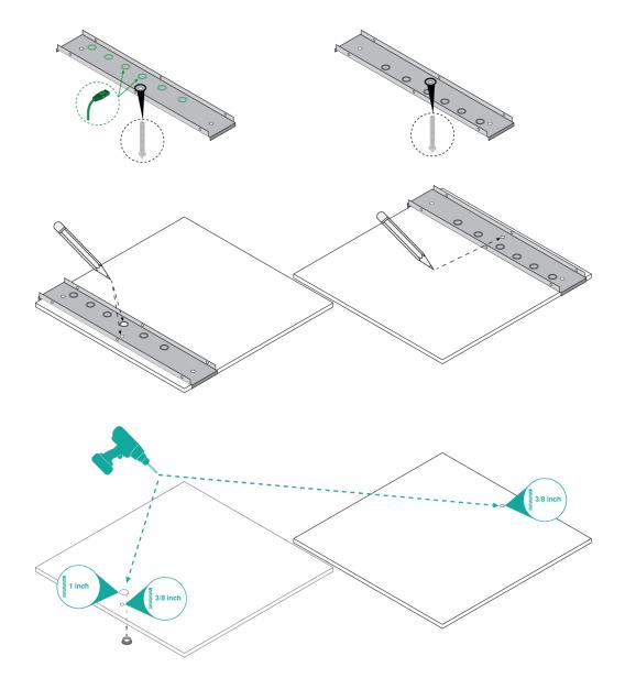
3. Reinstall the ceiling tiles. Place the tile bridges on the T-bars and align them with the holes in the ceiling tiles. If required, connect conduit and pull the Ethernet cable through the ceiling tile.
