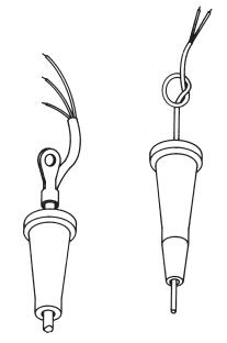
STRAIN RELIEF FOR ONE 6.4 mm (0.25 in.) CABLE
