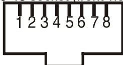
RJ-45 socket (front view):
