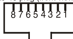
RJ-45 plug (front view):
