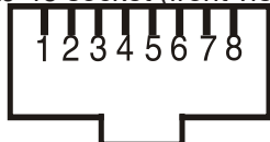
RJ-45 socket (front view):
