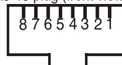
RJ-45 plug (front view):
