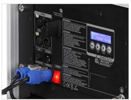
Address Setup – Use control menu to set DMX address. The machine occupies 3 control channels. The starting address is defined as the first channel from which the machine will respond to the controller. Always double check to make sure there are no overlapping channels in order to control the machine correctly.
