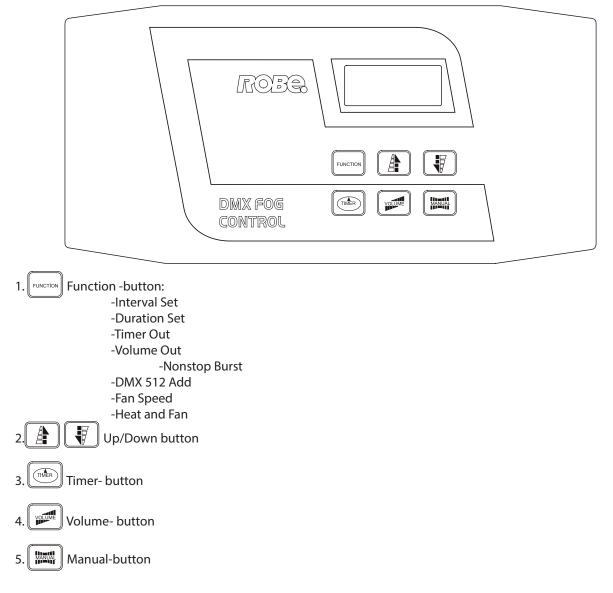
Wired multi-function remote control module with 5-pin XLR connector for ROBE Faze 1050 FT. Its interface allows the operator to customize fog machine functions by adjusting fogging duration, interval and volume. Its LCD displays current operating parameters, which are automatically stored in non-volatile memory, allowing the machine to be powered down without losing function settings. See instructions below:
