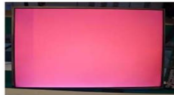
Vertical Block Source TAB IC Defect
