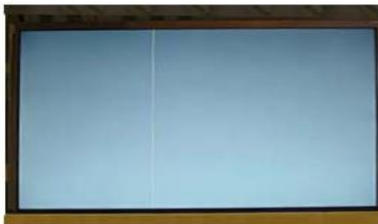
Vertical Line Source TAB IC Defect
